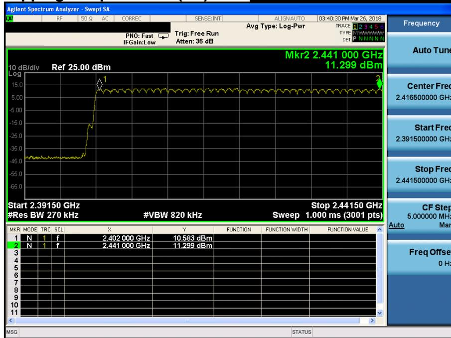
**Number of Hopping Frequencies 2(FH) *Hopping mode : Enable & 8DPSK***
