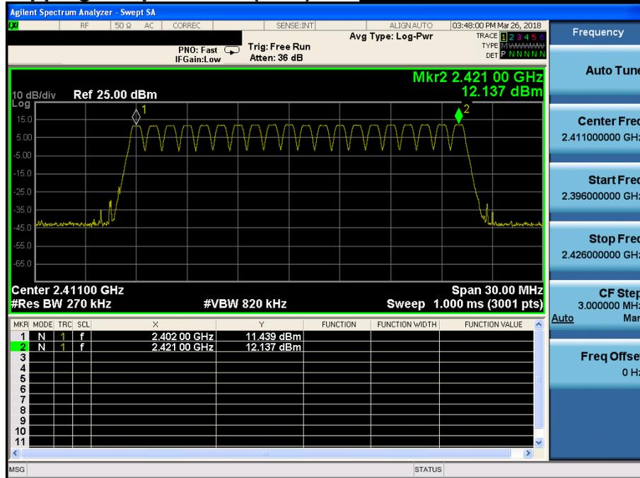
**Number of Hopping Frequencies 1(AFH)      *Hopping mode : Enable & π/4DQPSK***
