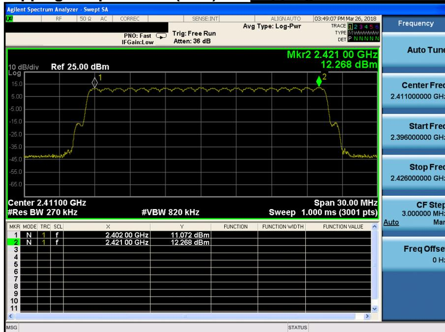
Number of Hopping Frequencies 1(AFH) *Hopping mode : Enable & 8DPSK*
