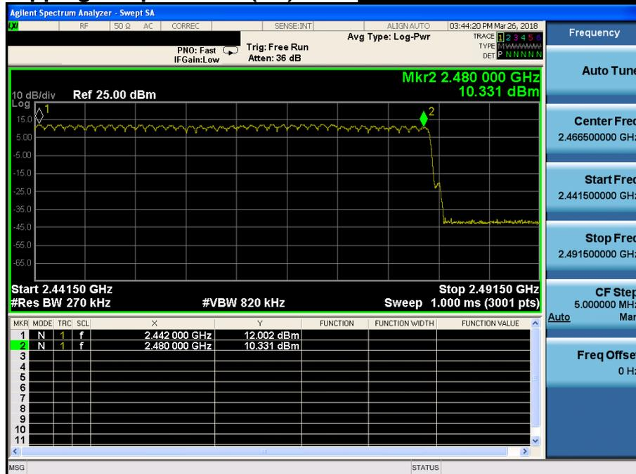
**Number of Hopping Frequencies 1(FH) *Hopping mode : Enable & 8DPSK***
