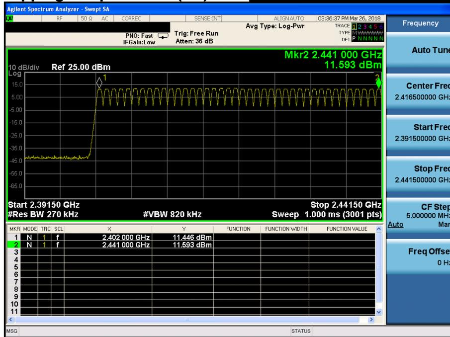
**Number of Hopping Frequencies 2(FH) *Hopping mode : Enable & GFSK***
