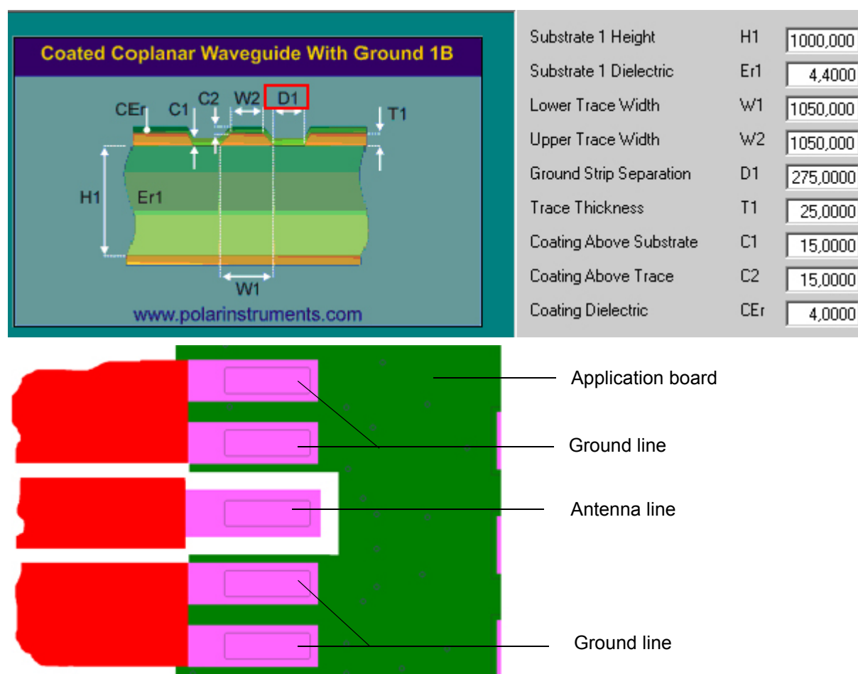
Figure 8: Micro-Stripline on 1.0mm Standard FR4 PCB - example 2
