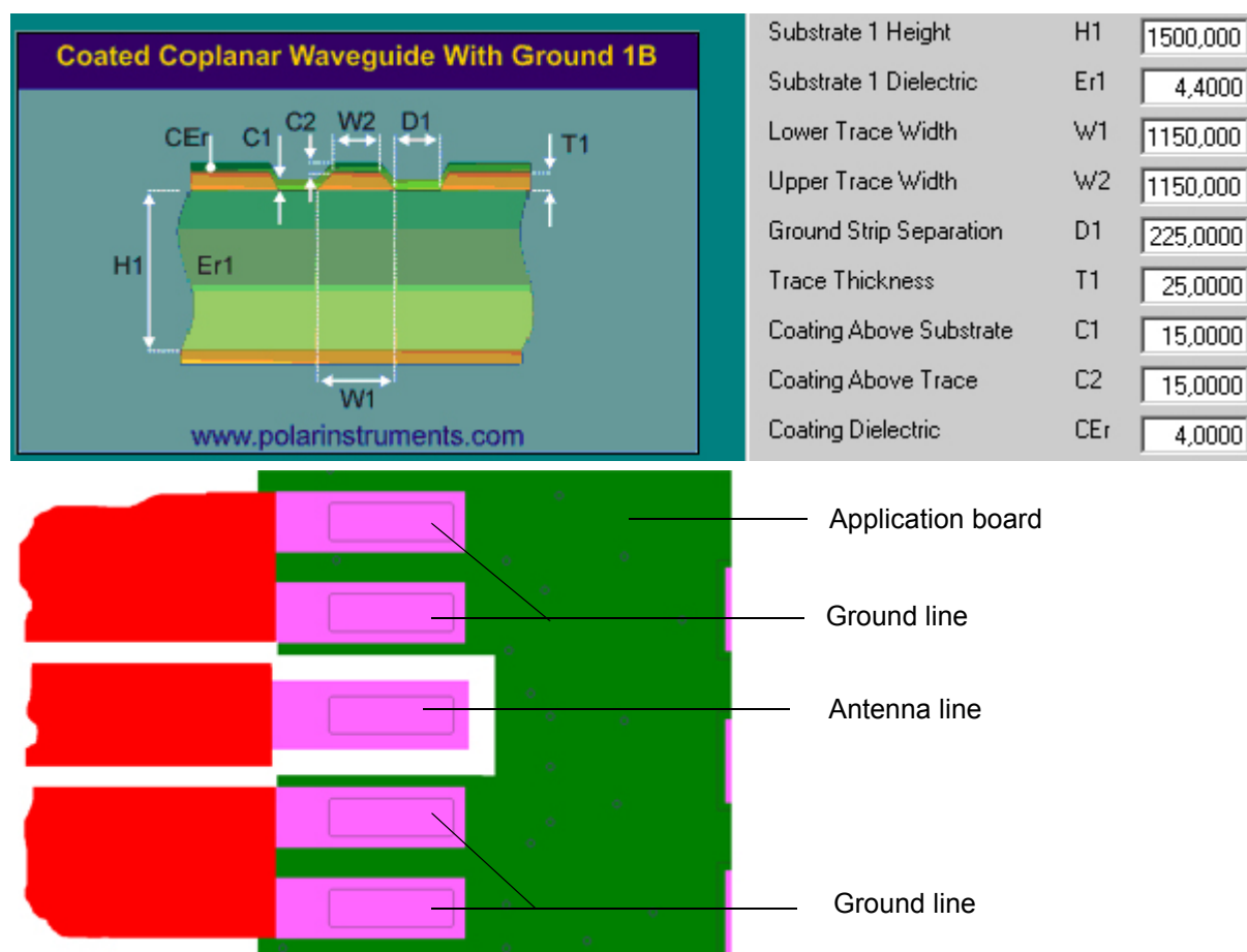
Figure 10: Micro-Stripline on 1.5mm Standard FR4 PCB - example 2
