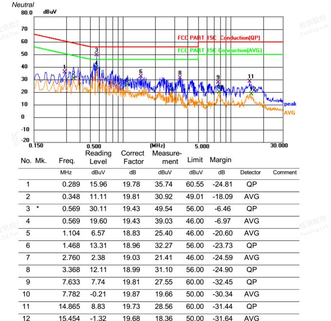
\*\*\*Note: Pre-scan all modes and recorded the worst case results in this report. Measurement= Reading + Correct Factor, Margin = Measurement – Limit. Correct Factor=Lisn Factor+Cable Factor+Insertion loss of Pulse Limiter
