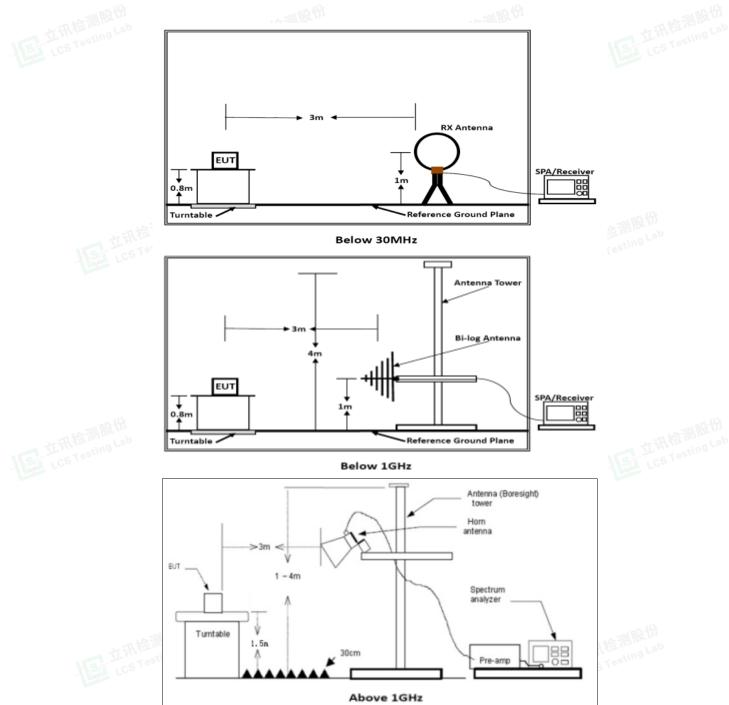
Above 18 GHz shall be extrapolated to the specified distance using an extrapolation factor of 20 dB/decade form 3m to 1m.
