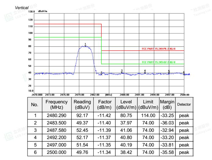
Note: Due to the measure PK emission level less than the AV limit value. No necessary to take down the AV emission level.
