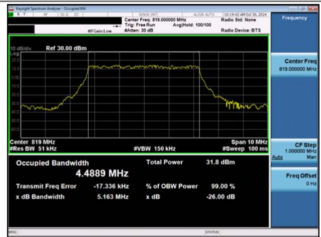
NTNV-n26(814-824)-PC3-15-5-M-DFT-BPSK-Outet1-PASS
