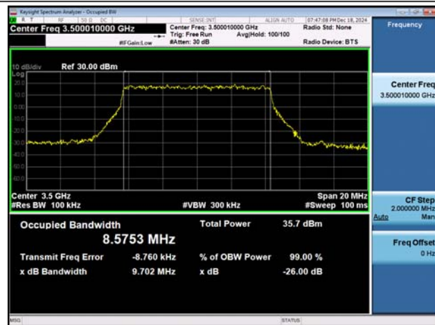
NTNV-n78(3450-3550)-PC2-30-10-M-DFT-QPSK-Out_ Full -Ant1-PASS
