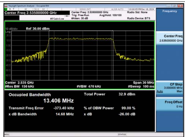
NTVN-n7-PC3-15-15-M-DFT-QPSK-Outter_Full-Ant1-PASS
