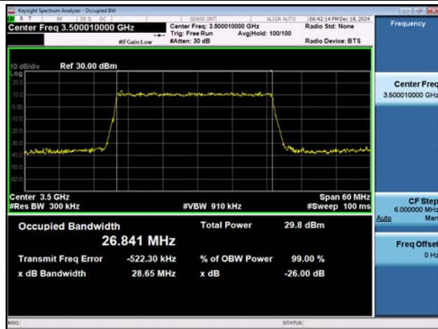
NTNV-n77(3450-3550)-PC3-30-30-M-DFT-QPSK-Outter_Full-Ant1-PASS
