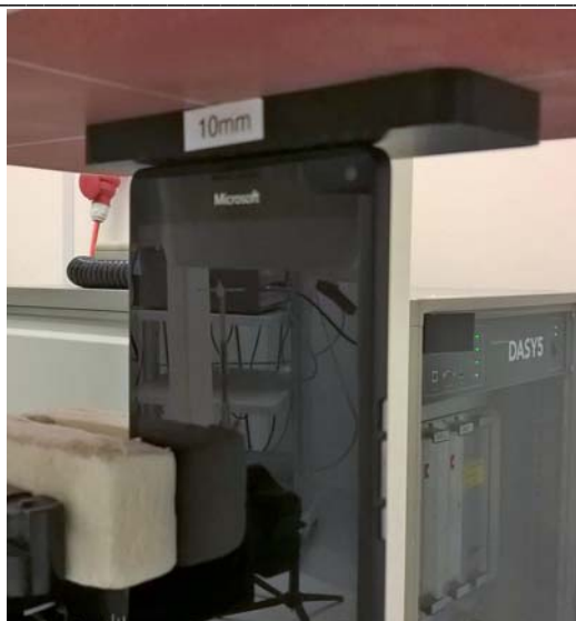
Photo of the device positioned for WR mode measurement – top edge facing phantom. The spacer was removed before the start of the measurements.
