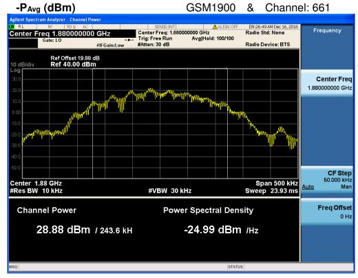
$PAPR (dB) = P_{Pk} (dBm) - P_{Avg} (dBm) = 29.23 dBm - 28.88 dBm = 0.35 dB$
