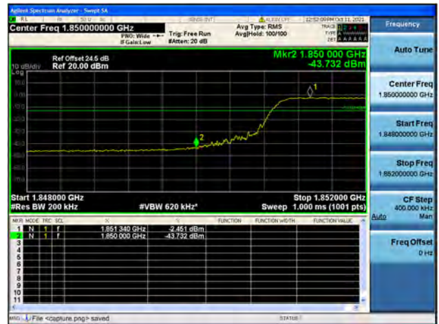
Band25 / 20MHz / High CH / QPSK / FULL RB
