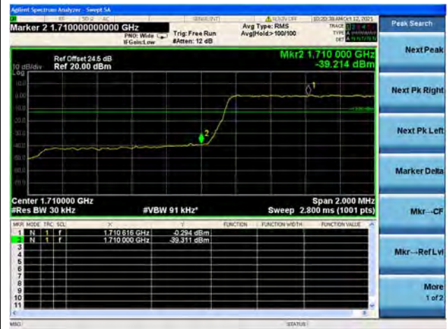
Band66 / 1.4MHz / High CH / QPSK / FULL RB
