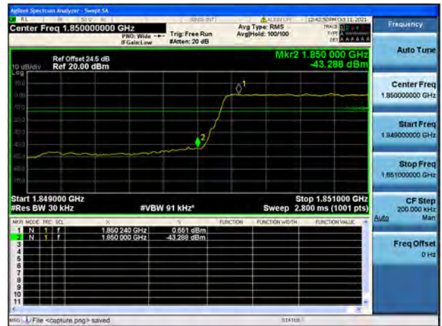
Band25 / 1.4MHz / High CH / QPSK / FULL RB
