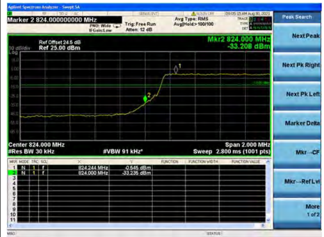
Band26 / 3MHz / High CH / QPSK / FULL RB
