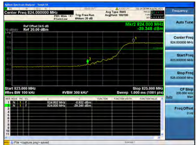
Band5 / 10MHz / High CH / QPSK / FULL RB
