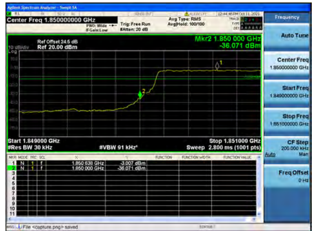
Band25 / 3MHz / High CH / QPSK / FULL RB
