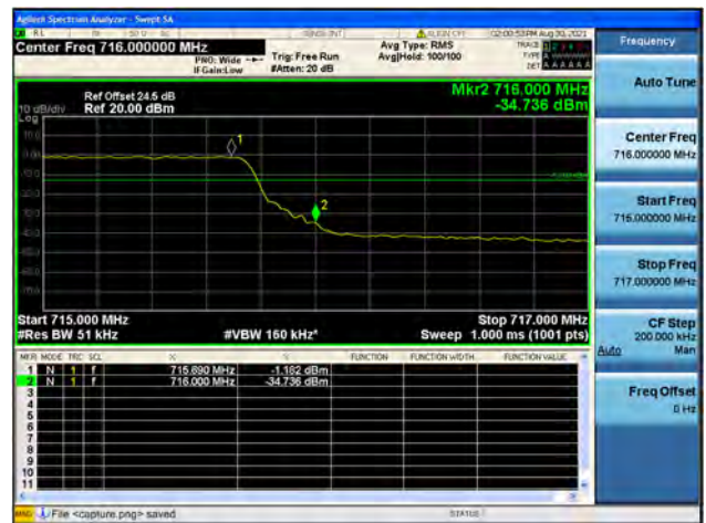
Band12 / 5MHz / High CH / QPSK / FULL RB
