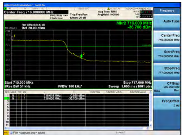
Band17 / 5MHz / High CH / QPSK / FULL RB
