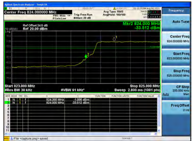
Band5 / 3MHz / High CH / QPSK / FULL RB
