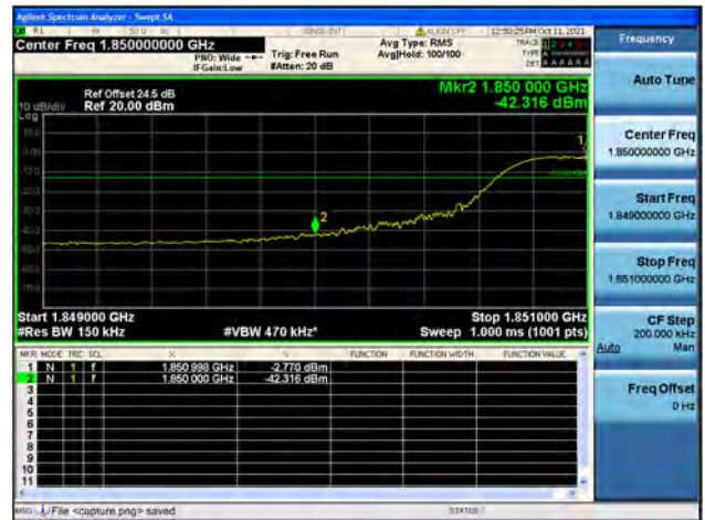
Band25 / 15MHz / High CH / QPSK / FULL RB
