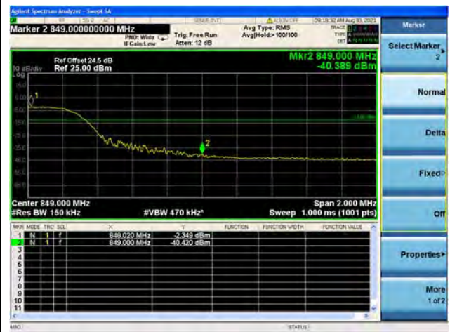
Band26 / 15MHz / High CH / QPSK / FULL RB
