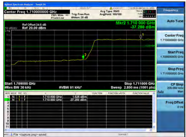
Band4 / 1.4MHz / High CH / QPSK / FULL RB
