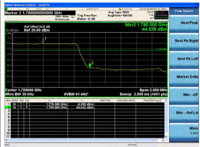
Band66 / 1.4MHz / High CH / QPSK / FULL RB
