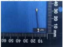
2.4G WIFI&BT(2400-2500MHz) antenna gain is -0.49dBi 5G WIFI(5000-6000MHz) antenna gain is 3.65dBi
