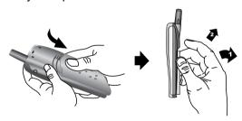
NOTE: If the battery is not correctly placed in the battery compartment, the handset will not turn on and/or the battery may detach during use.
