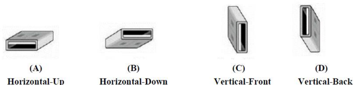
F-3. USB Connector Orientations Implemented on Laptop Computers
