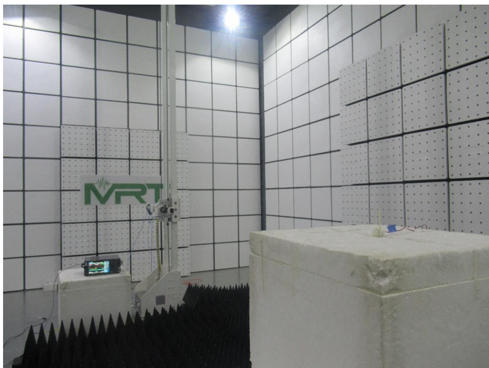
Photograph 4: Set-up photo for Radiated Spurious Emission, 18GHz ~ 40GHz
