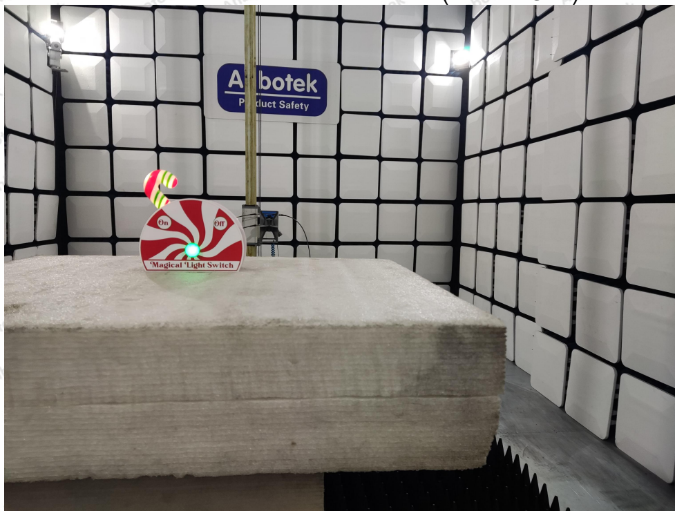
Photo of Radiation Emission Test (above 1GHz)
