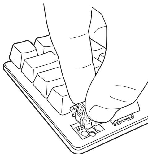
Note: Be sure to align the new keyswitch properly before insertion to prevent bent pins or damage.
