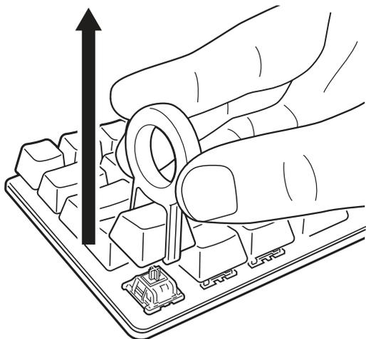
2. Position the tips of the keyswitch puller (I) under the keyswitch top and bottom tabs, then press in and lift to remove.
