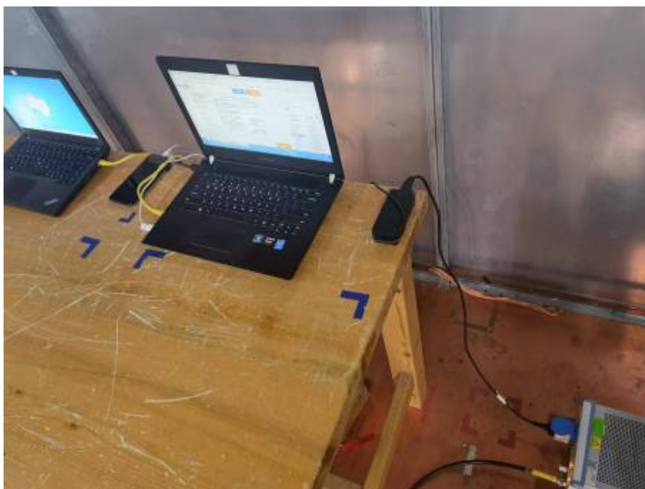
Conducted Emissions Test Setup (with laptop)
