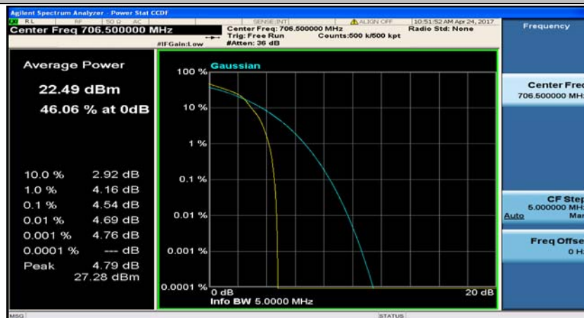
(Channel Bandwidth: 5 MHz)_LCH_16QAM_12RB#0
