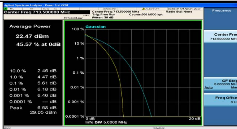
(Channel Bandwidth: 5 MHz)_HCH_QPSK_25RB#0
