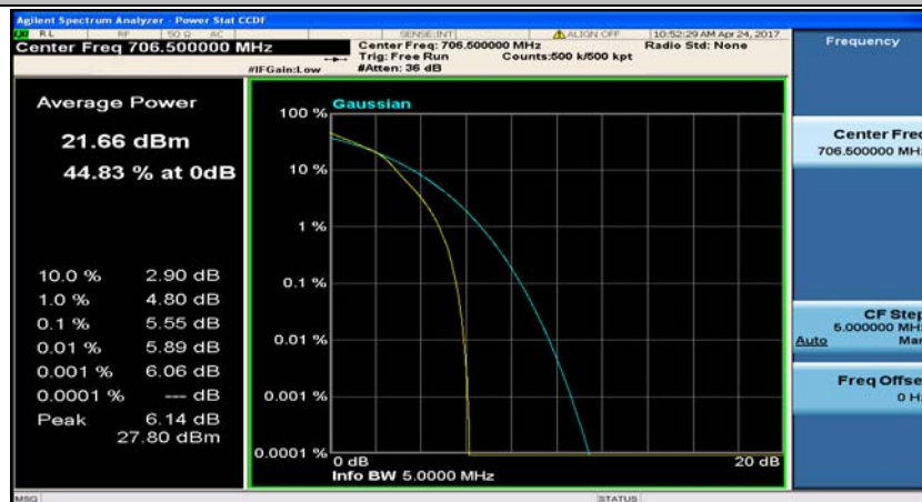
(Channel Bandwidth: 5 MHz)_LCH_16QAM_25RB#0
