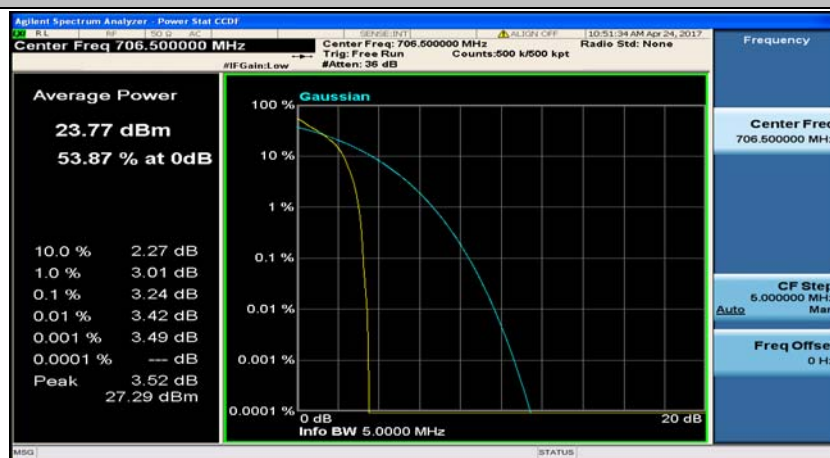
(Channel Bandwidth: 5 MHz)_LCH_QPSK_12RB#0
