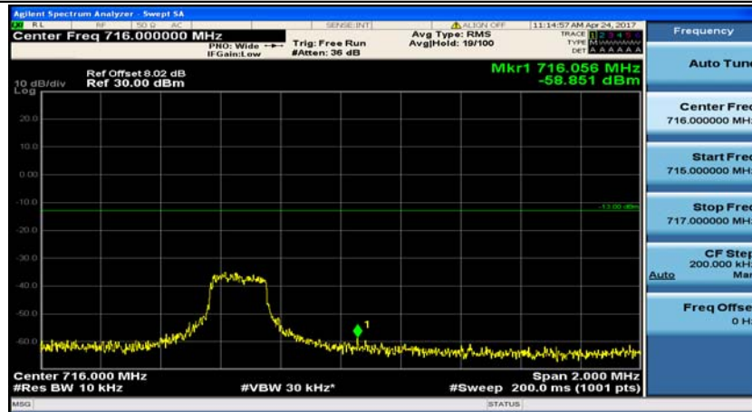
(Channel Bandwidth: 5 MHz)_HCH_16QAM_1RB#12
