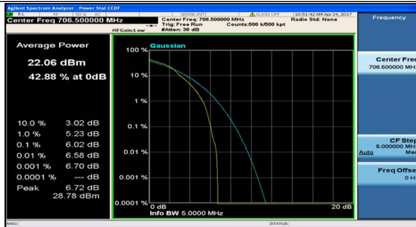
(Channel Bandwidth: 5 MHz)_LCH_16QAM_1RB#12
