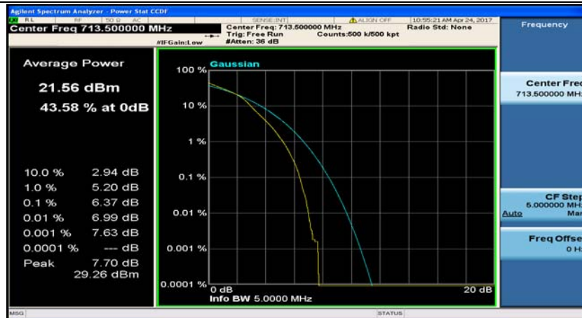
(Channel Bandwidth: 5 MHz)_HCH_16QAM_12RB#13
