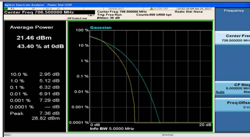
(Channel Bandwidth: 5 MHz)_LCH_16QAM_12RB#6
