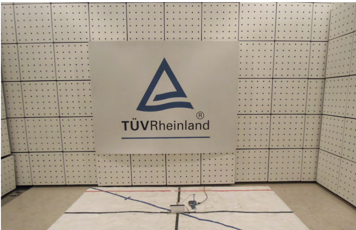
Photograph 7: Set-up for Spurious Emissions (Front view 1) - RFMTA331215IMAB701-ANT
