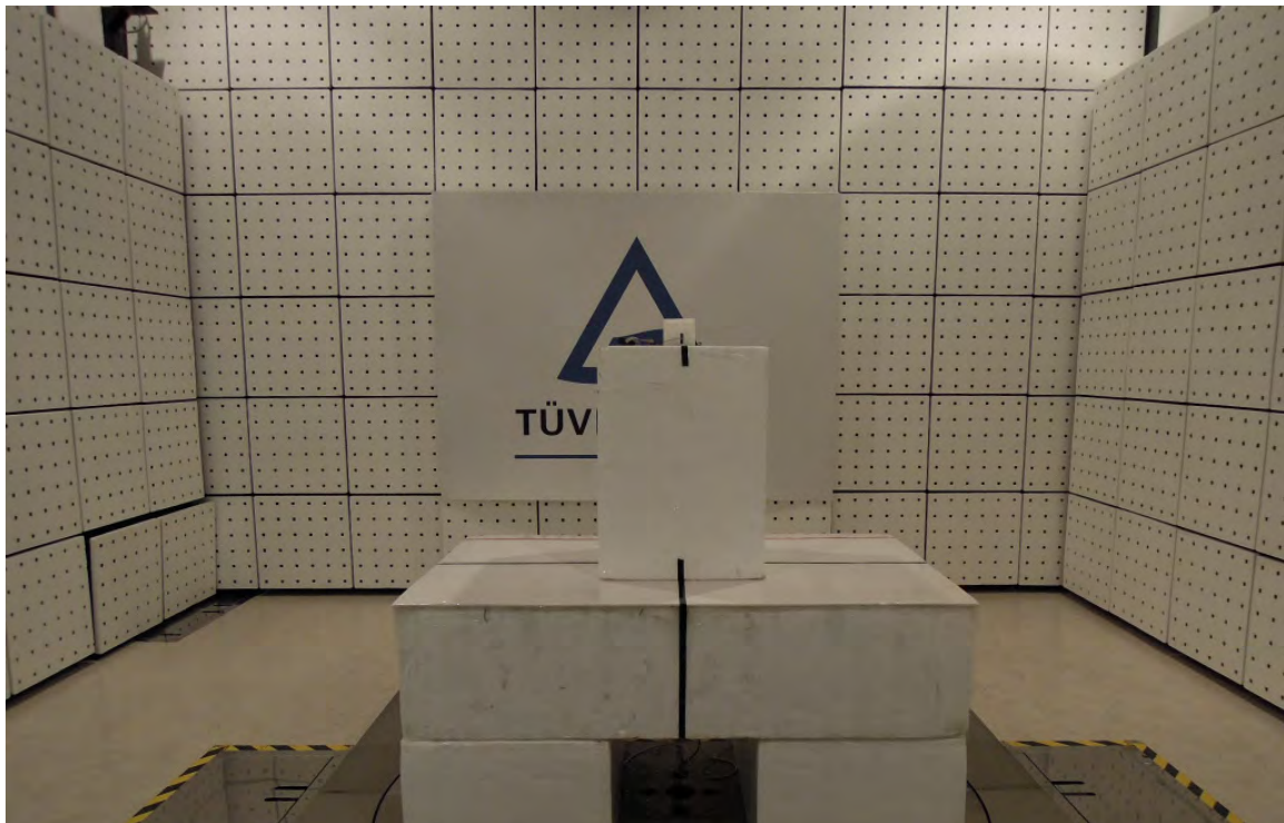
Photograph 23: Set-up for Spurious Emissions (Front View)- 14615300100 -ANT
