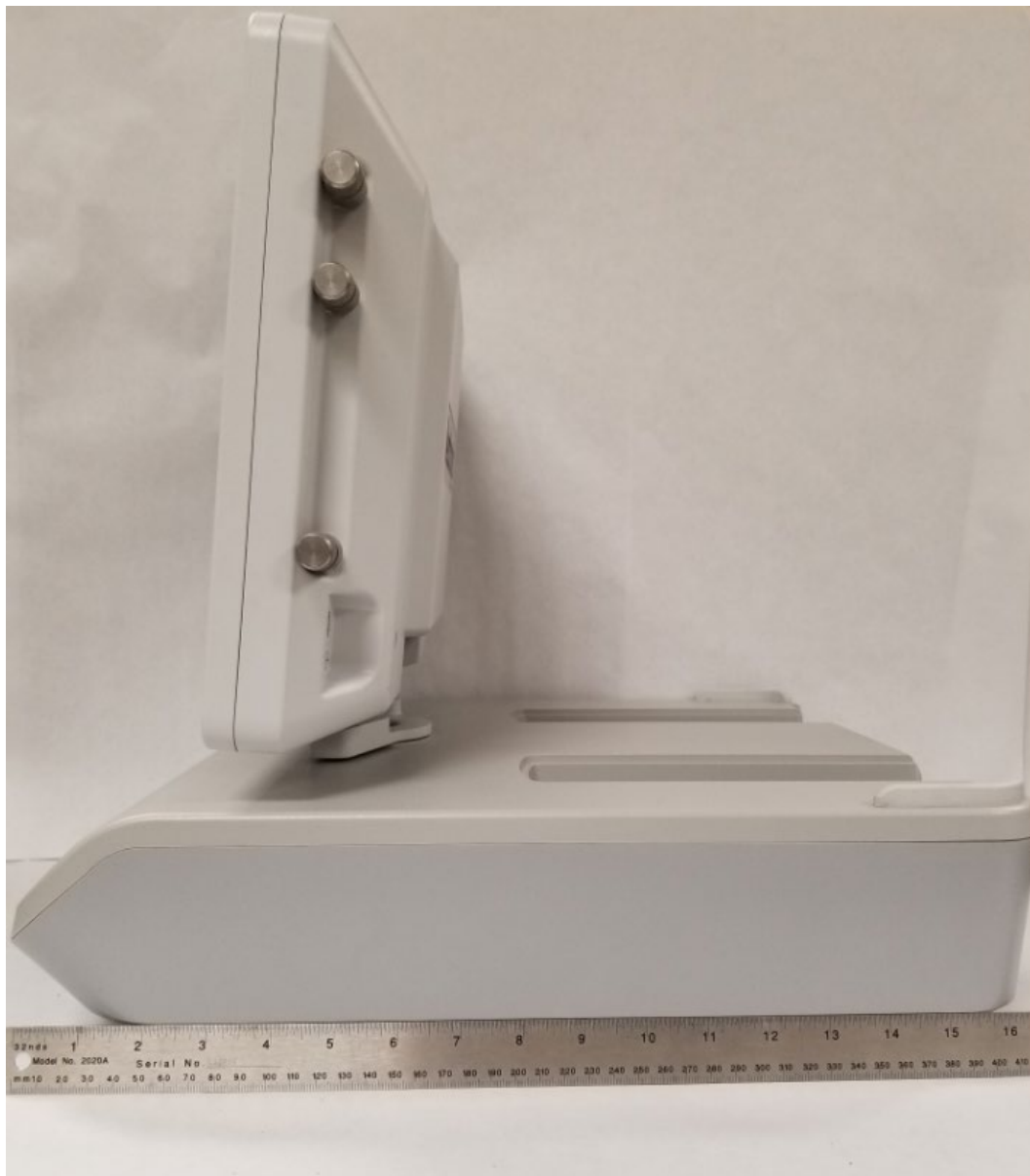
Figure 4: NIM Vital Console, Model NIM4CM01, Right Side View Base (Length) with dimensions
