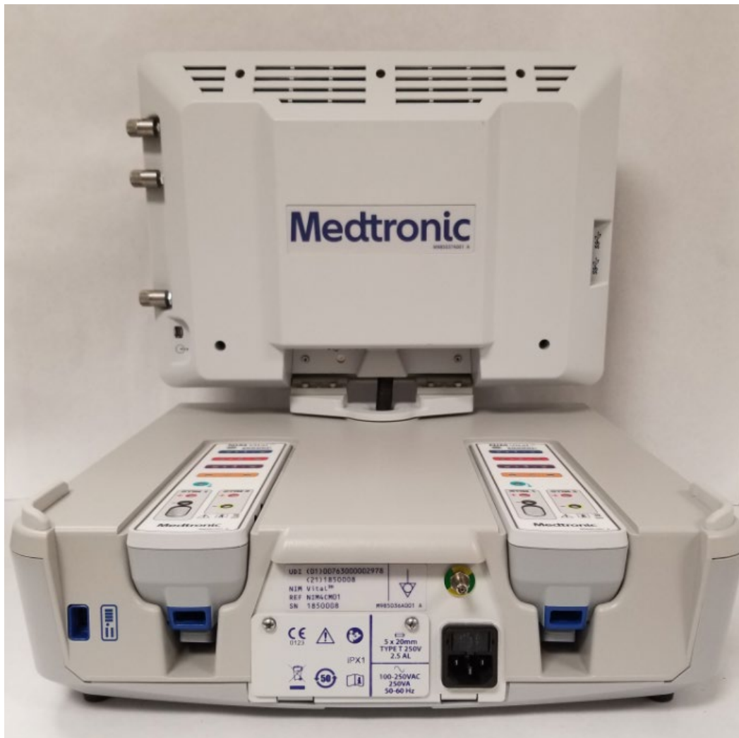
Figure 4 NIM Vital Console, Model NIM4CM01, Rear View including Patient Interfaces
