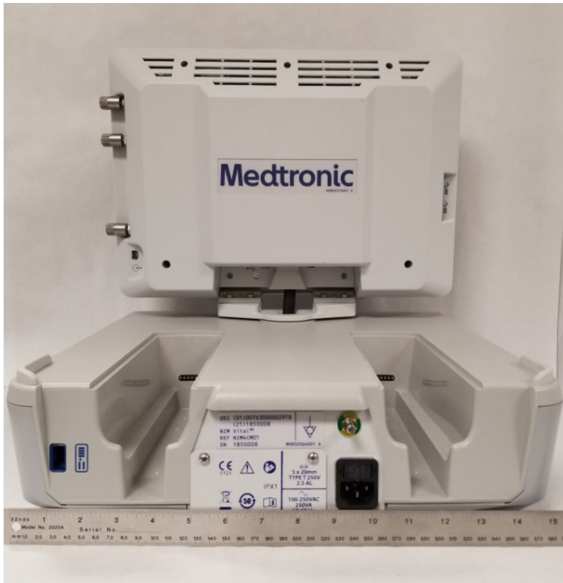
Figure 3 NIM Vital Console, Model NIM4CM01, Rear View (Width) with dimensions
