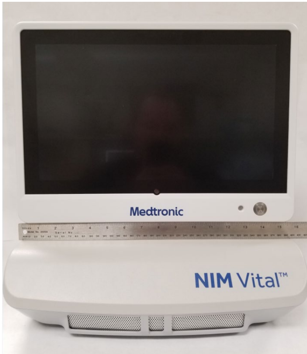
Figure 2 NIM Vital Console, Model NIM4CM01, Front View Screen (Width) with dimensions
