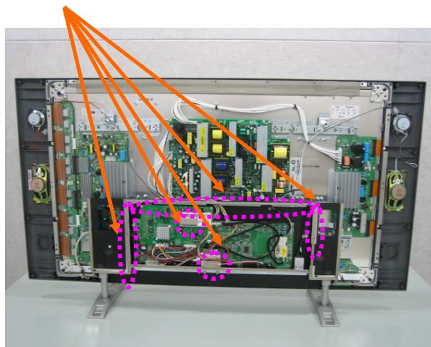
**3. Apply a ferrite Core to the Speaker cable**
