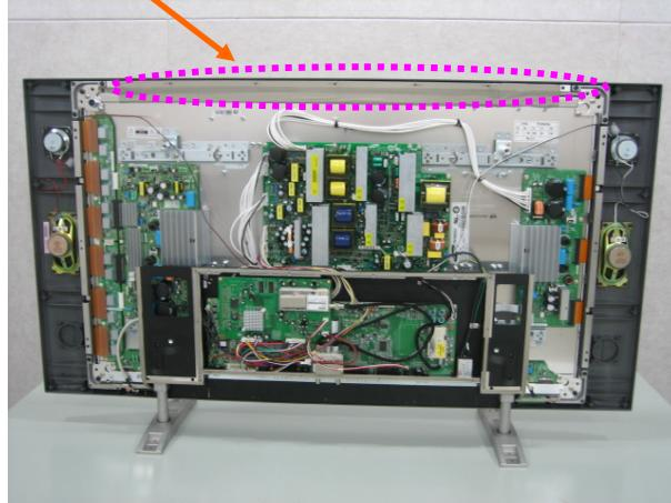
**2. Attach a gasket on TV Tuner and Board Bracket**
