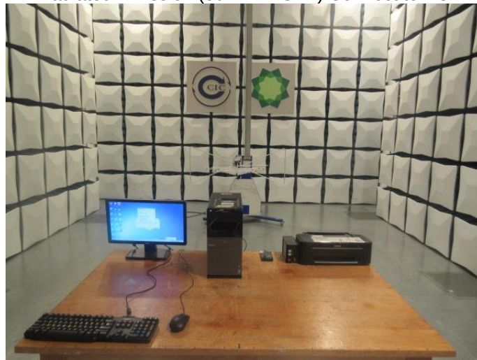
Radiated Emission (above 1GHz) Connect to PC
