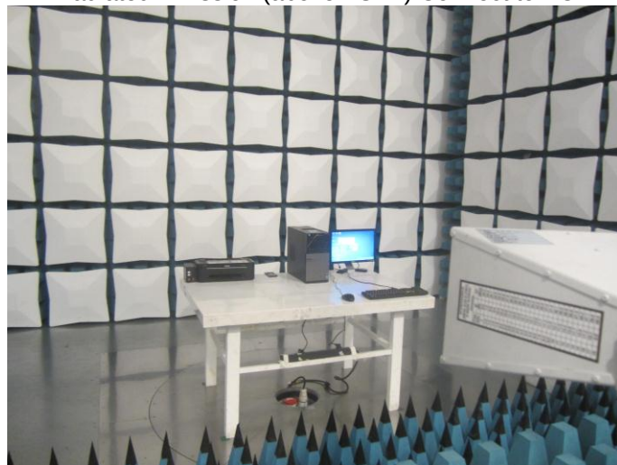
Radiated Emission (above 1GHz) Connect to PC
