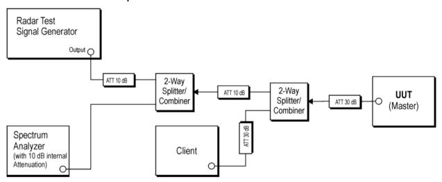
Remark: During the test, a lower radar signal level -60dBm was used.
