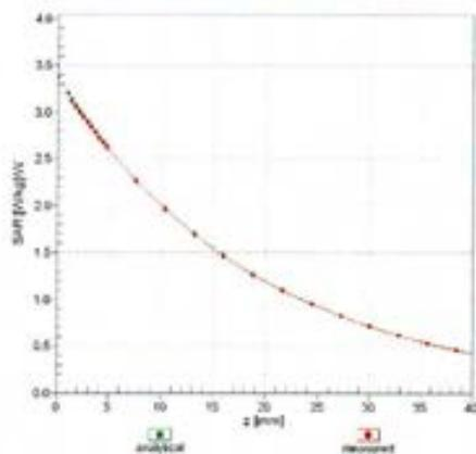
$f = 2450 \text{ MHz}, \text{WG}LS R22 (H_{convF})$
