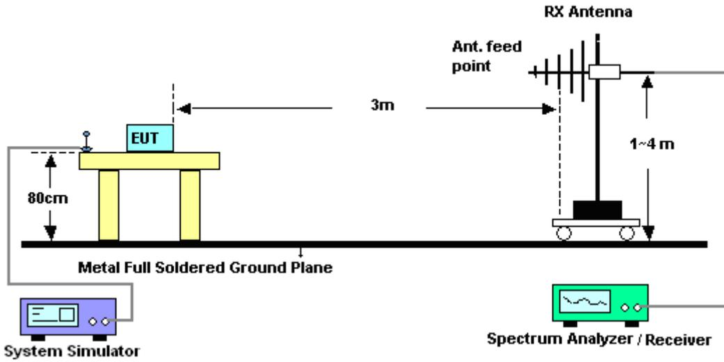
For radiated test above 1GHz
