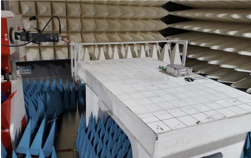
Figure C3. High Range Radiated Emission test setup 18-40GHz
