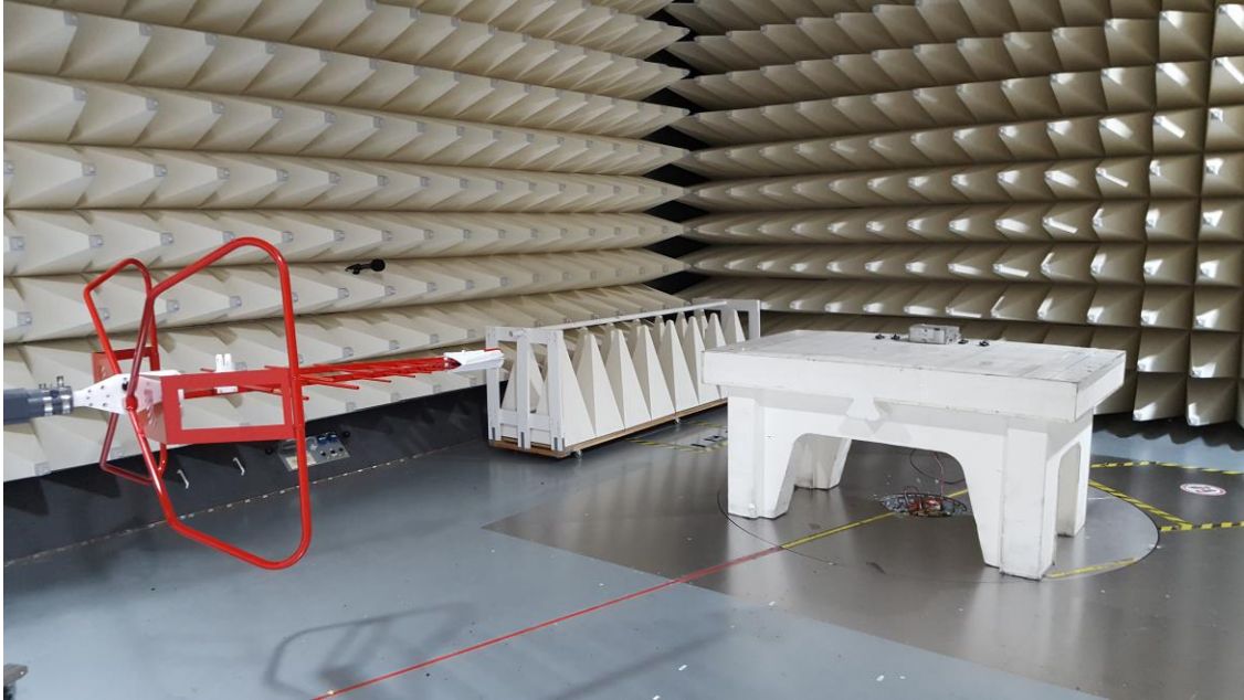
Figure C1. Low Range Radiated Emission test setup
