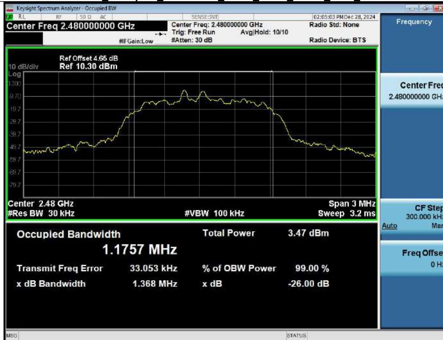
99% Occupied Bandwidth NVNT_ANT1_2-DH1_2480_00
