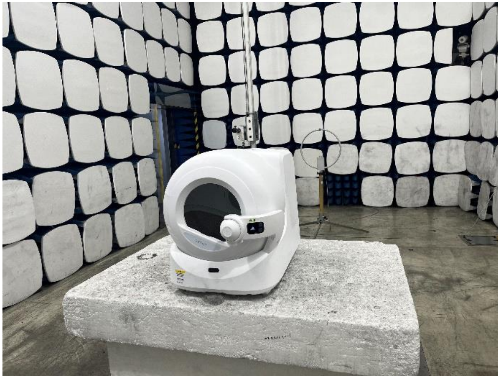
NFC (Setup Photo--Below 30MHz)
