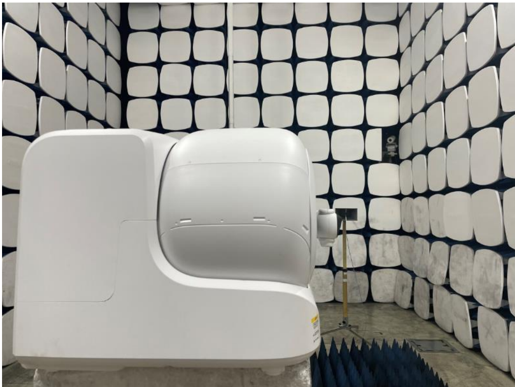
1.4 Set-up for Spurious Emissions above 1GHz
