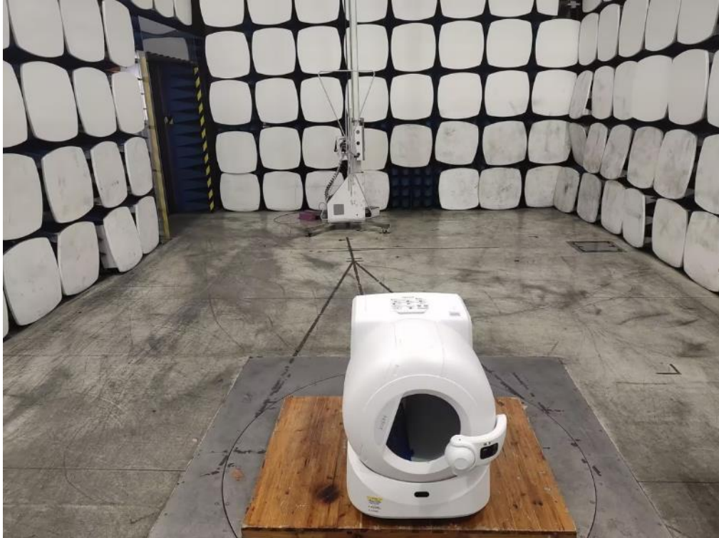
1.4 Set-up for Spurious Emissions above 1GHz
