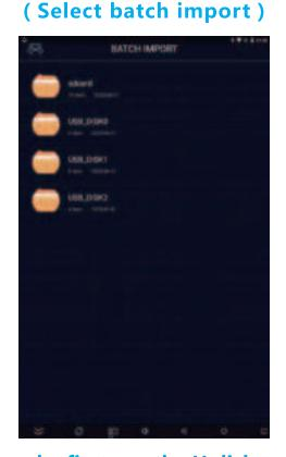
Batch registration: in batch registration mode, first use the U disk to name the employee's picture (such as "Zhang San. JPG") under a folder. Then click the batch import function on the face recognition machine. Select the picture folder under the U disk to import.
