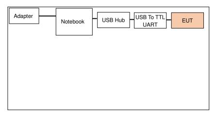
Test Configuration: Radiated Emission
