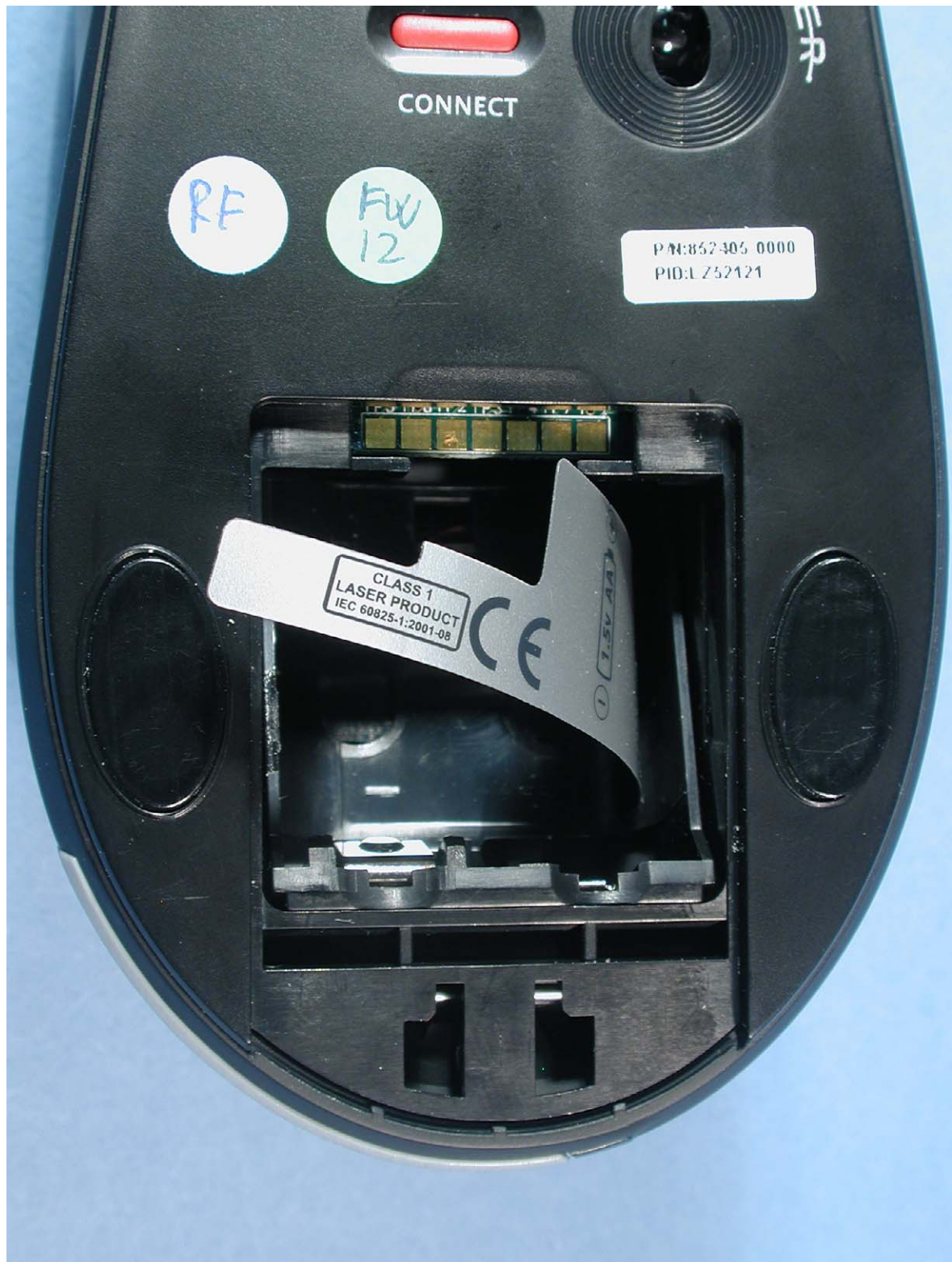
Photograph 3: Battery compartment of M-RAZ105
