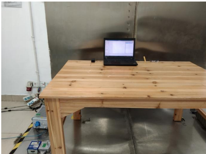
Conducted Emission Setup Front View
