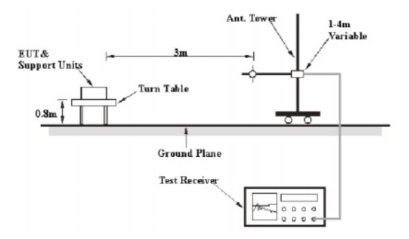
The radiated emission tests were performed in the 3 meters test site, using the setup accordance with the FCC MP - 5. The specification used was the FCC part 18.
