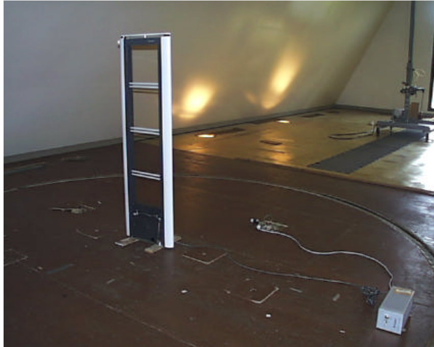
Photo 3 -- Strata PX Radiated Emissions Test Setup -- Front View
