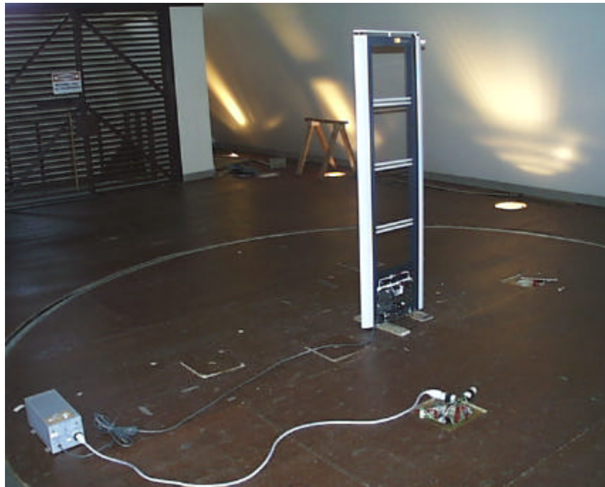
Photo 4 -- Strata PX Radiated Emissions Test Setup – Rear View
