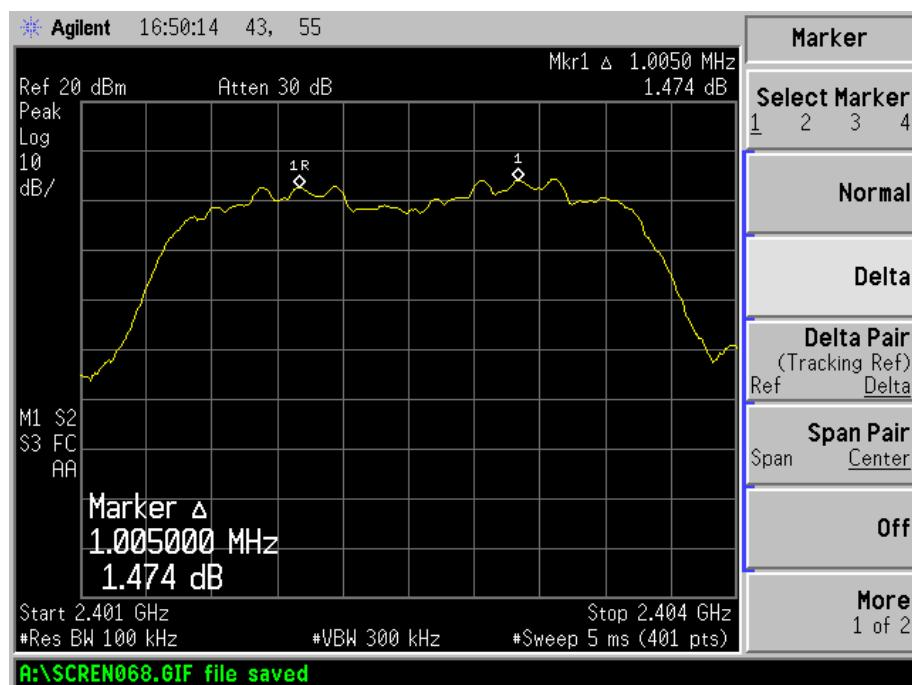
Channel Spacing (Middle CH=1MHz)
