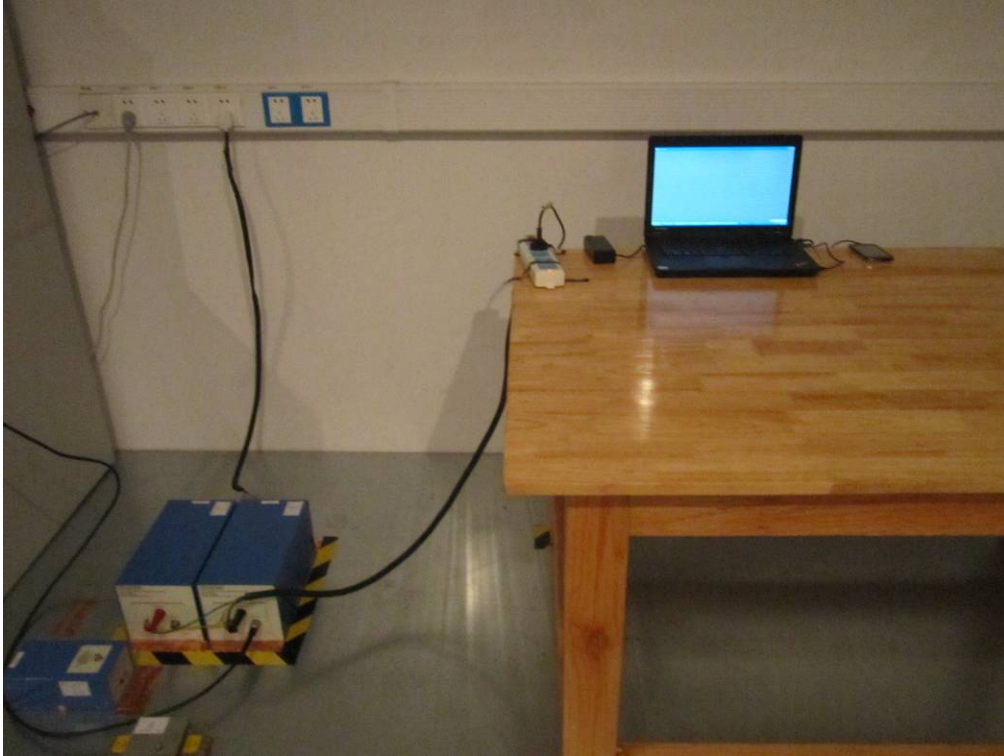
Conducted Emissions Test Setup Front View
