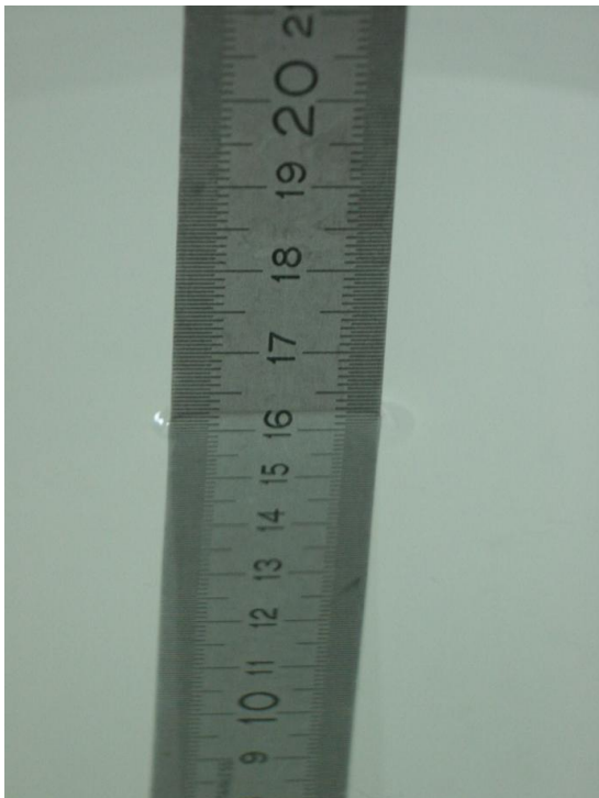
Fig. 16: Liquid depth for WCDMA IV Body measurements.
