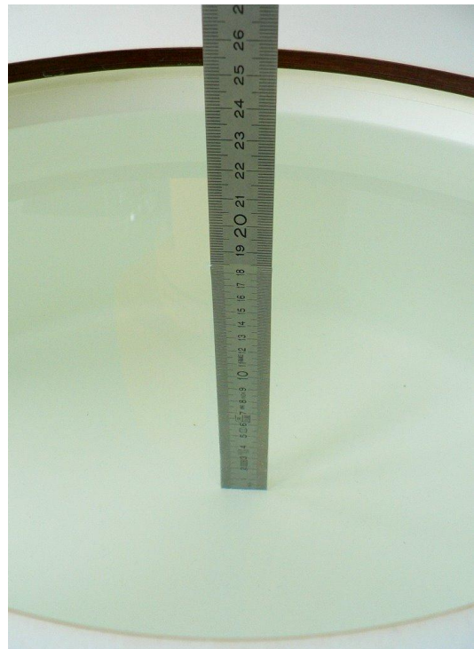
Fig. 15: Liquid depth for GPRS 1900 and WCDMA II Body measurements.
