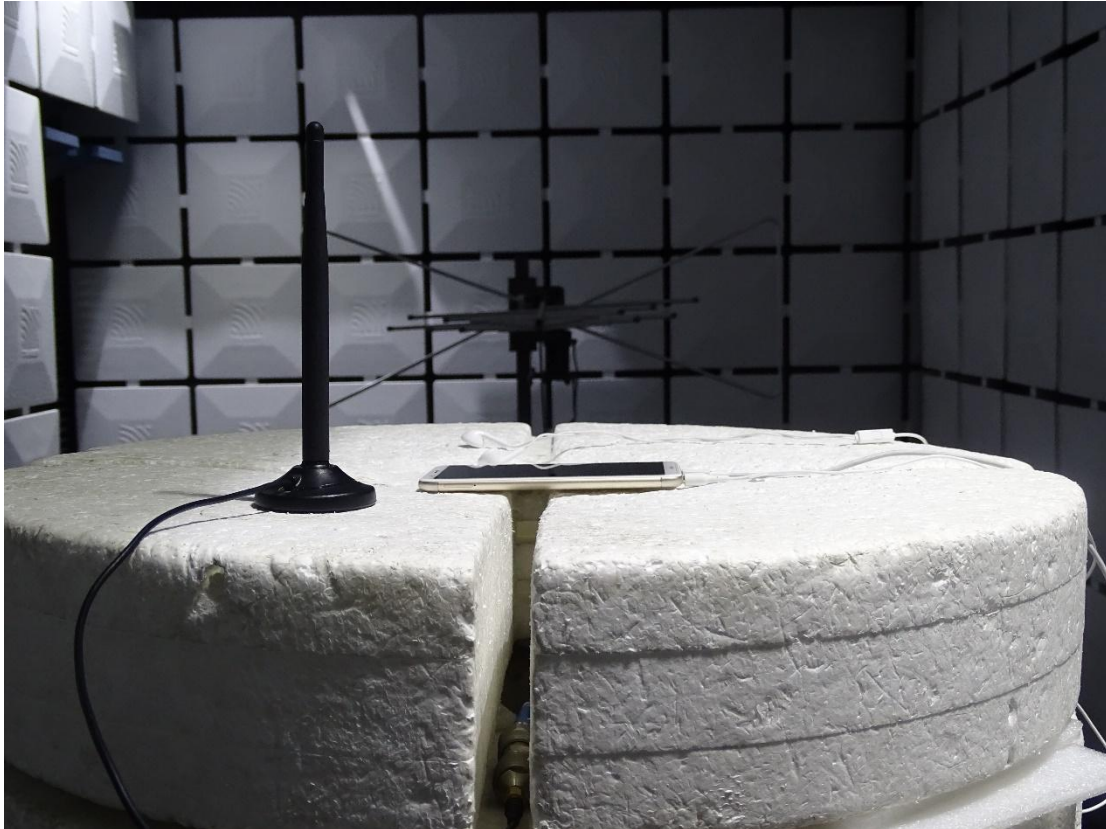
Radiated Spurious Emission (below 3GHz)
