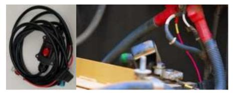
Connect the positive terminal to the normally open contact of the relay, and the negative terminal to the negative electrode of the battery or the vehicle body.
