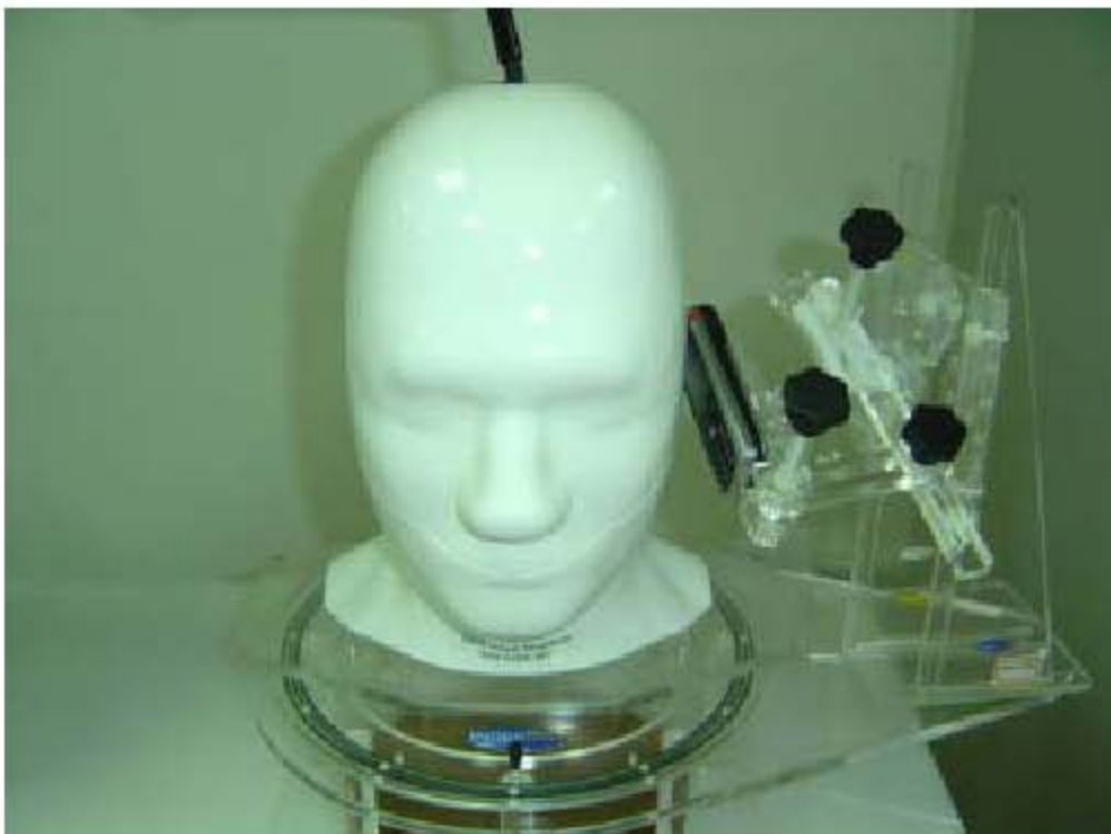
Fig.4 EUT Left Head Tilt15 Position
