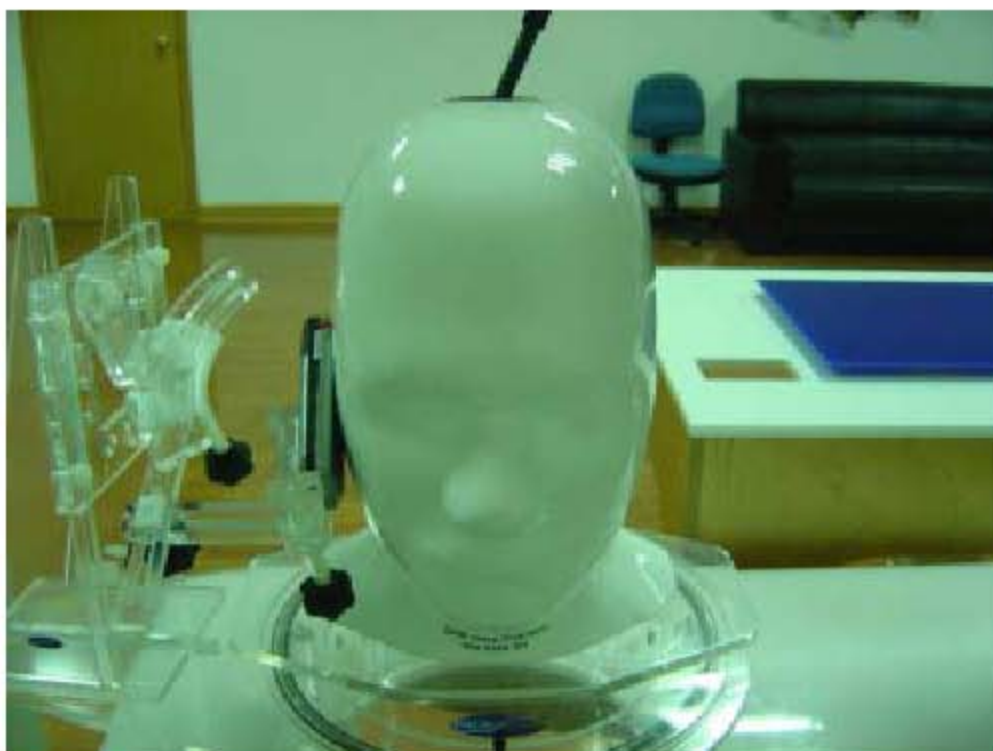
Fig.5 EUT Right Head Touch Cheek Position
