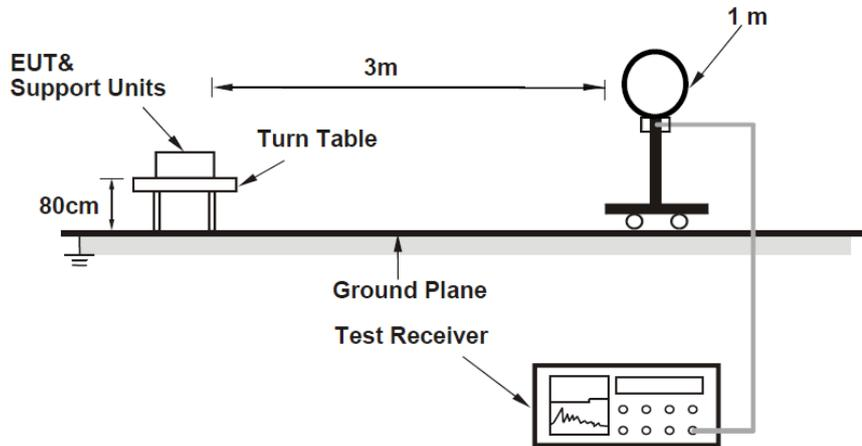
For Radiated emission 30MHz to 1GHz
