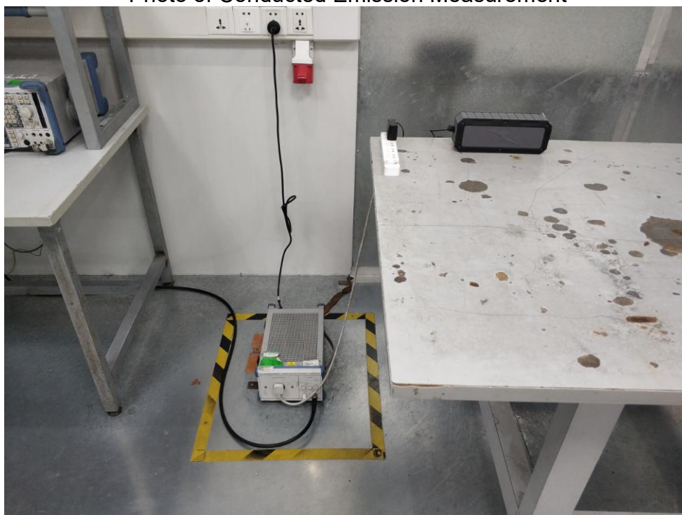
FCC ID: 2AJQ7-IJSP3013 Photo of Conducted Emission Measurement
