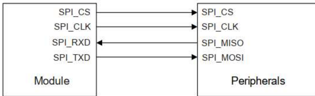
Figure 4-11: Reference Circuit of SPI Application
