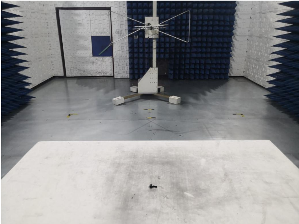
RADIATED EMISSION TEST SETUP ABOVE 1GHz
