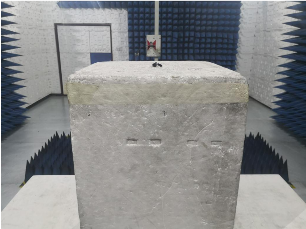
RADIATED EMISSION TEST SETUP ABOVE 1GHz
