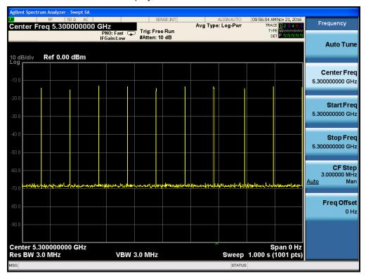
Time Display, WLAN Channel Traffic (Streaming Video)
