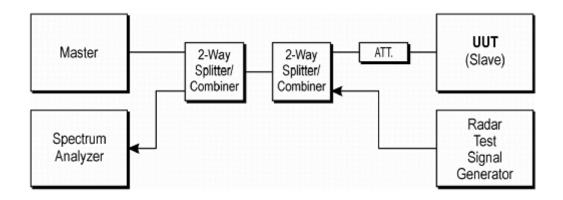
Figure 3-1. Conducted Test Setup for DFS
