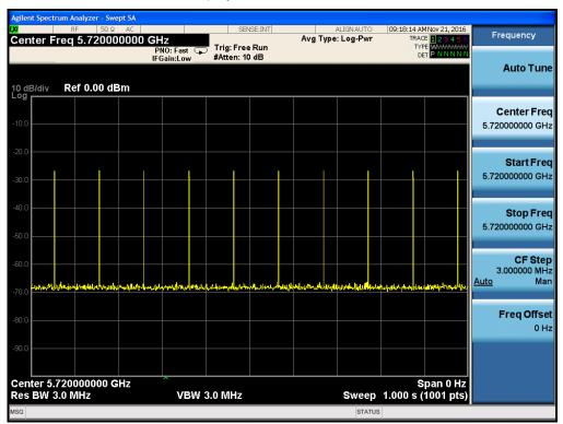
Time Display, WLAN Channel Traffic (Streaming Video)
