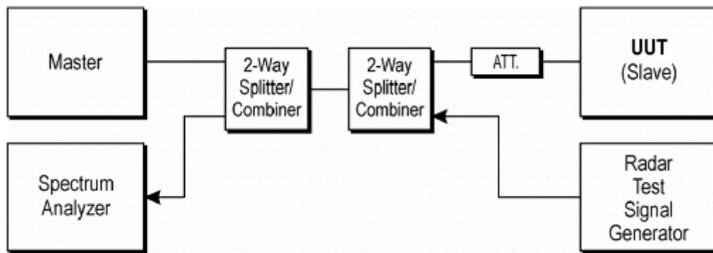
**Figure 3-1. Conducted Test Setup for DFS**
