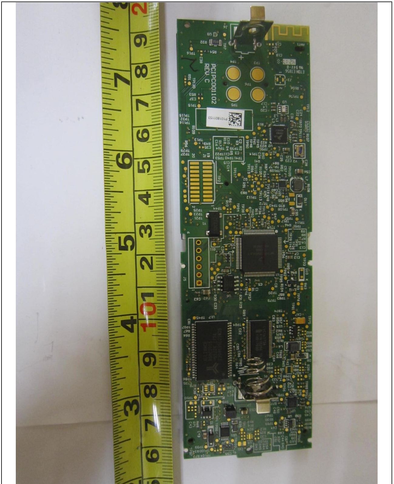
Main-Board PCB Trace Side
