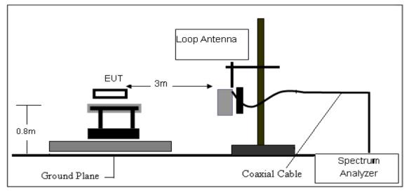
2. Radiated Emission Test-Up Frequency 30MHz~1GHz
