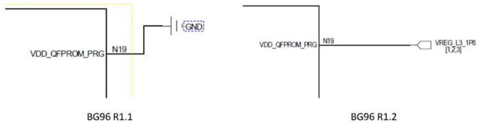
Figure 1: Schematic Designs of BG96 R1.1 and R1.2
