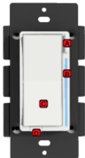
**A. Config Button:** This button is used to enter the configuration menu on your switch. When you hold it down for 10-15 seconds, the LED Bar (B) will light up Yellow to indicate you're in config mode. Then follow the config menu on Page 10 to configure your switch to the way you'd like.
