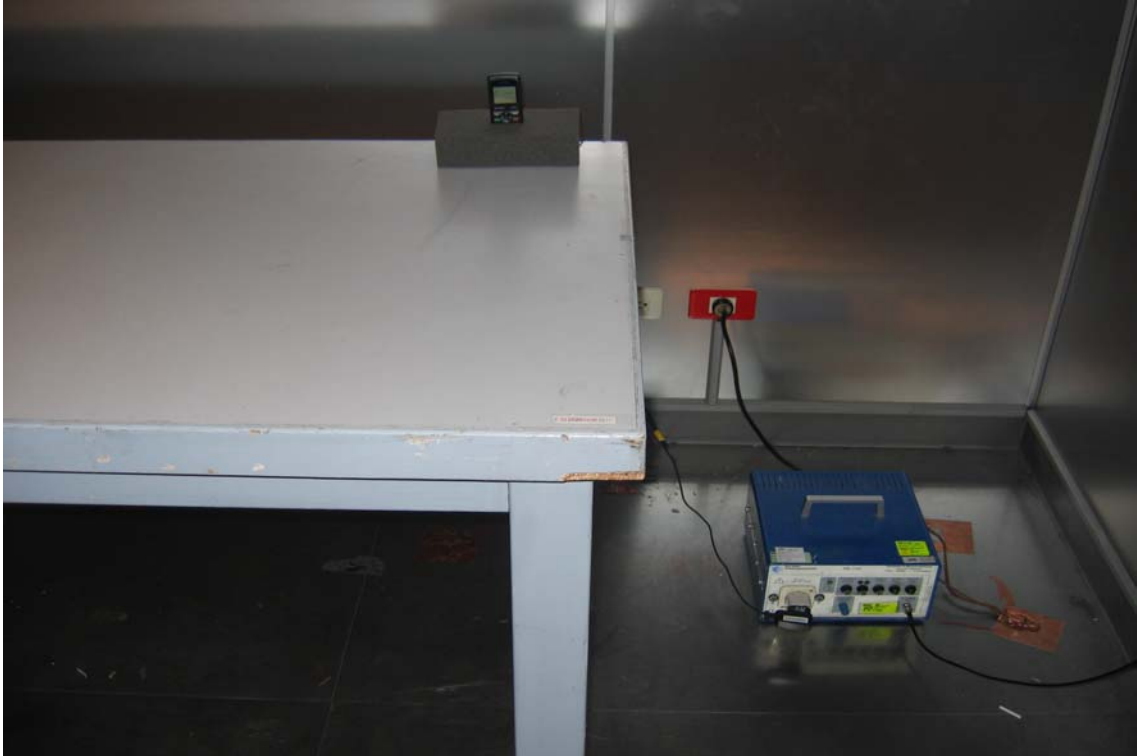
Conducted Emission Test Setup Photo(Power Adaptor)
