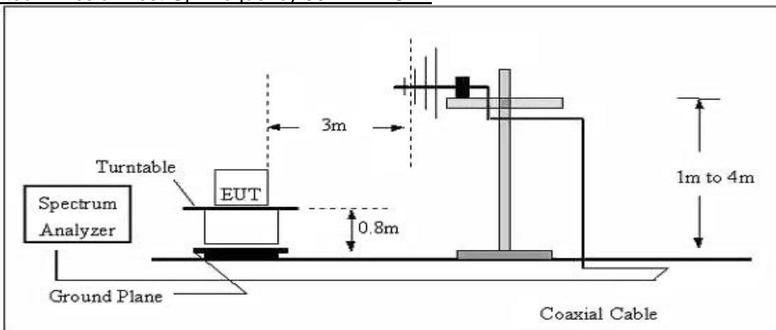
Radiated emission test-up frequency above 1GHz
