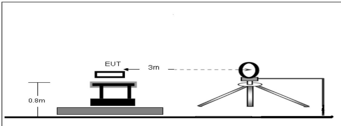
Radiated Emission Test-Up Frequency 30MHz~1GHz
