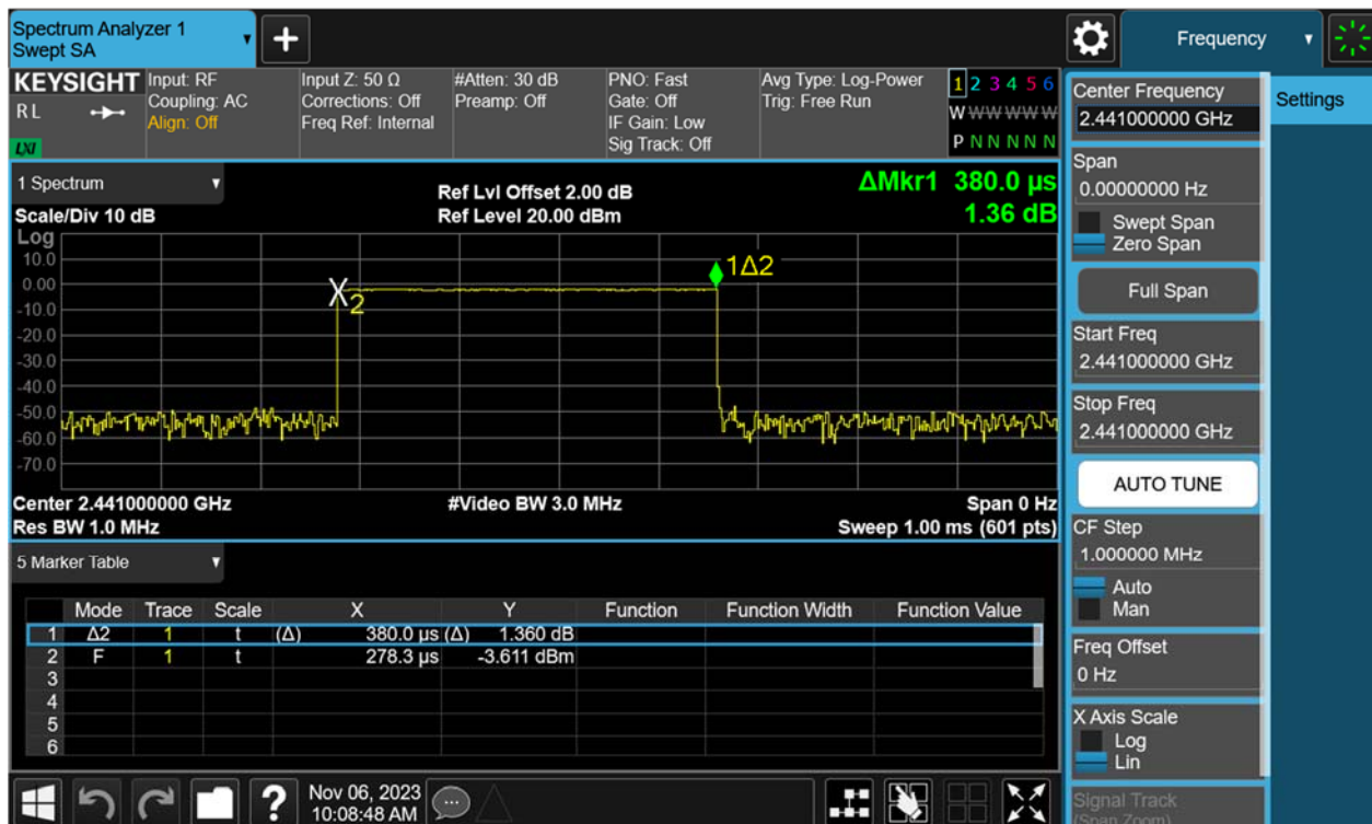
Figure 38: Time of Occupancy, 2441MHz, GFSK DH3
