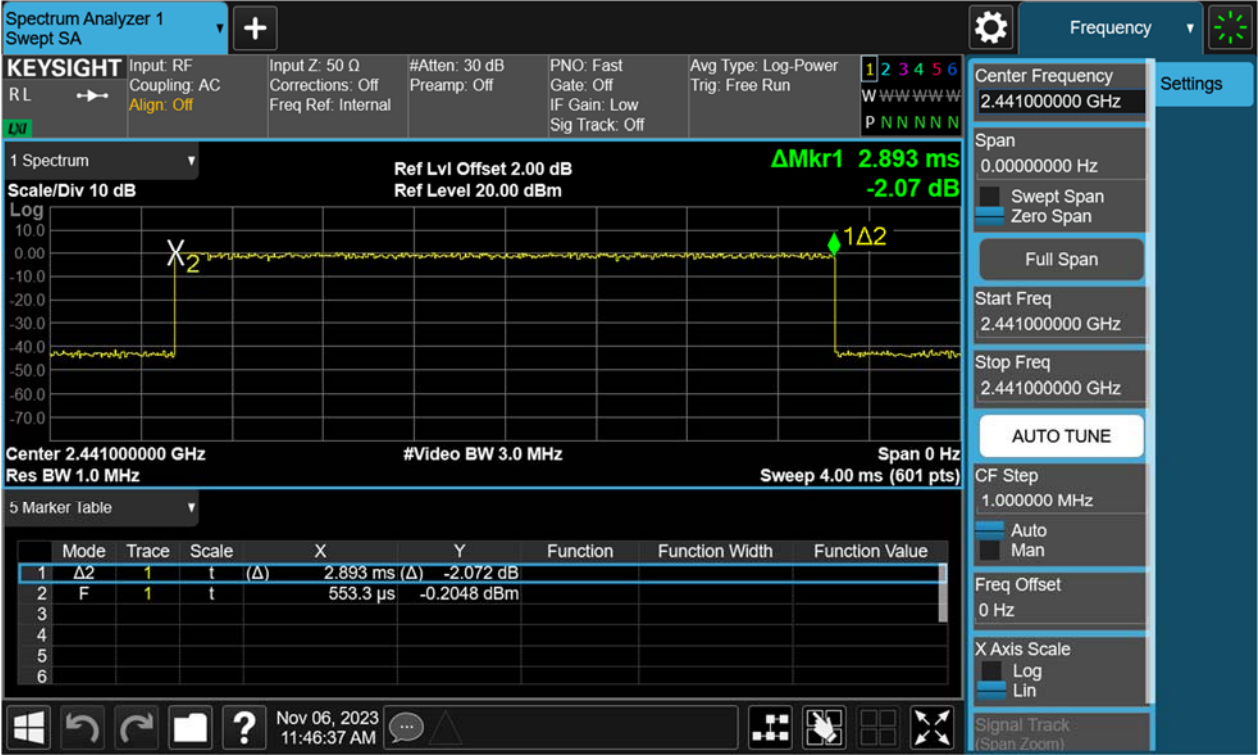
Figure 45: Time of Occupancy, 2441MHz, 8-DPSK DH5
