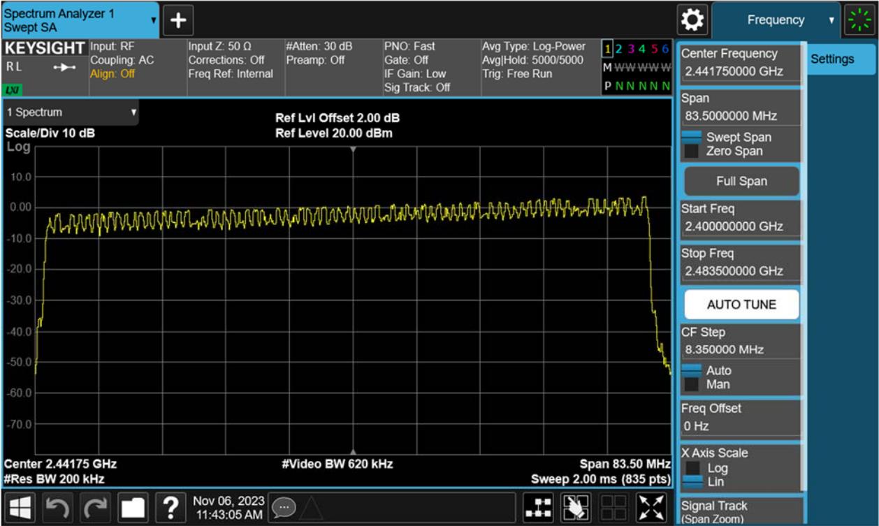
Figure 36: Number of Hopping Frequency, Hopping Mode, 8-DPSK
