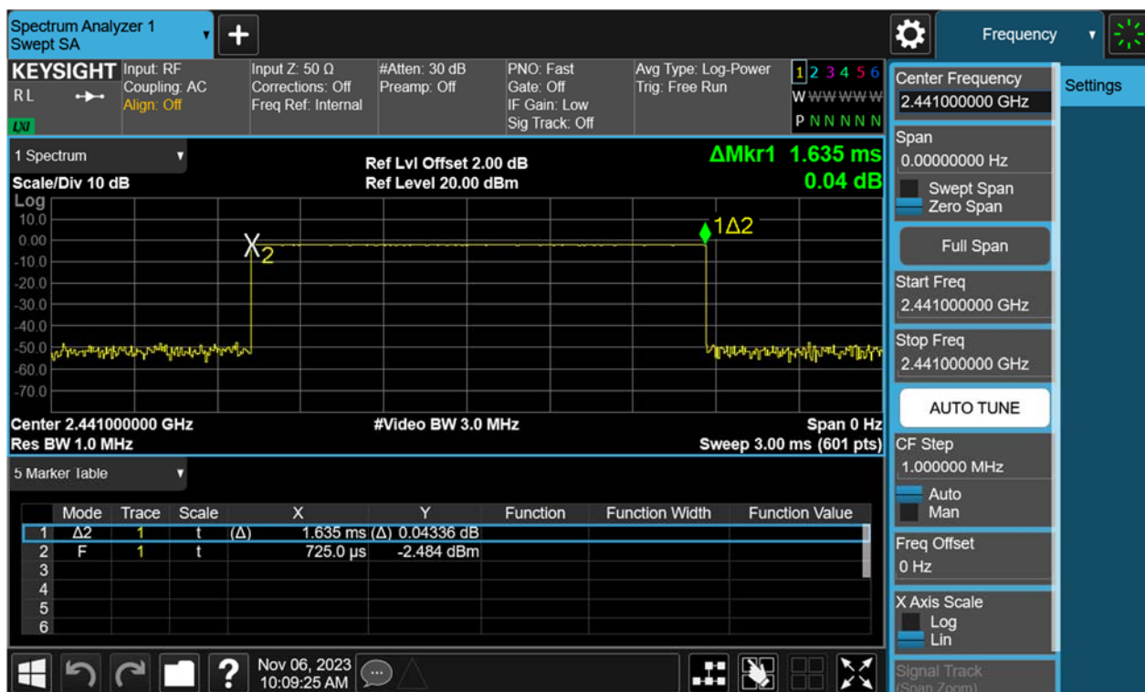
Figure 38: Time of Occupancy, 2441MHz, GFSK DH3
