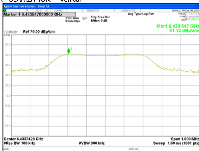
Plot 7.7.54 Radiated emission measurements at the seventh harmonic of high carrier frequency
